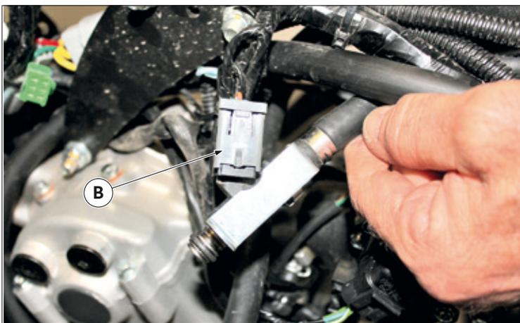
Disconnect the fuel injector connector "B".
