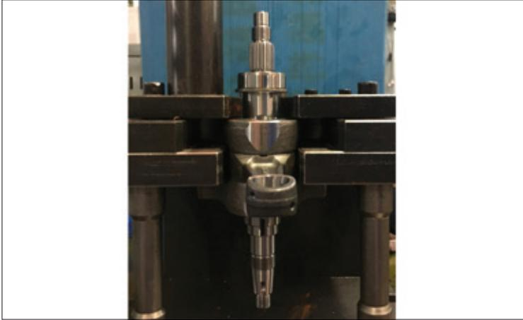
**13.8.3 Crankshaft bearing inner ring assembling**
