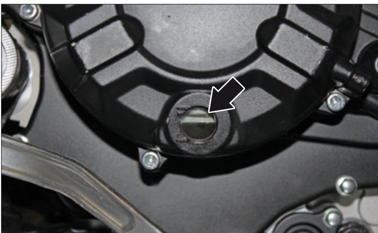
Measure 1500-1600 ml of oil with the measuring glass and fill the motor from the filling opening with the oil contained in the glass using a funnel before closing the oil cap.
