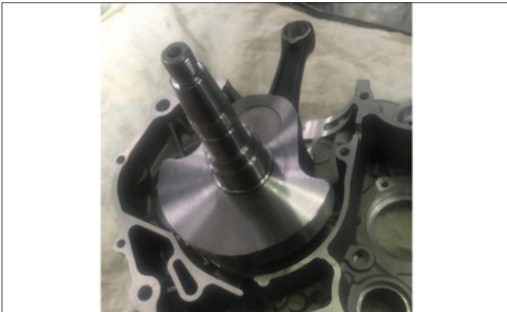
Install the crankshaft on the right half-crankcase to check that the shaft assembly is correct.
