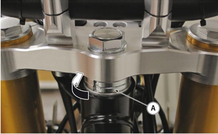
Loosen the 1st steering column fastening ring nut "A" 1/2 turn.
