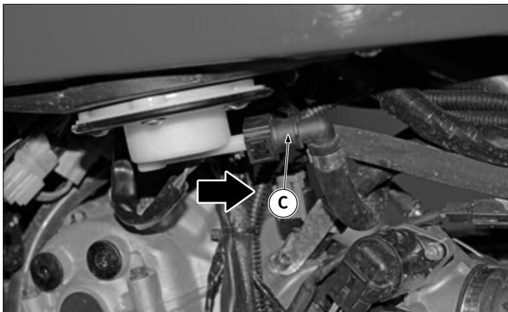
Disconnect the rubber tube "C" from the fuel pump.
