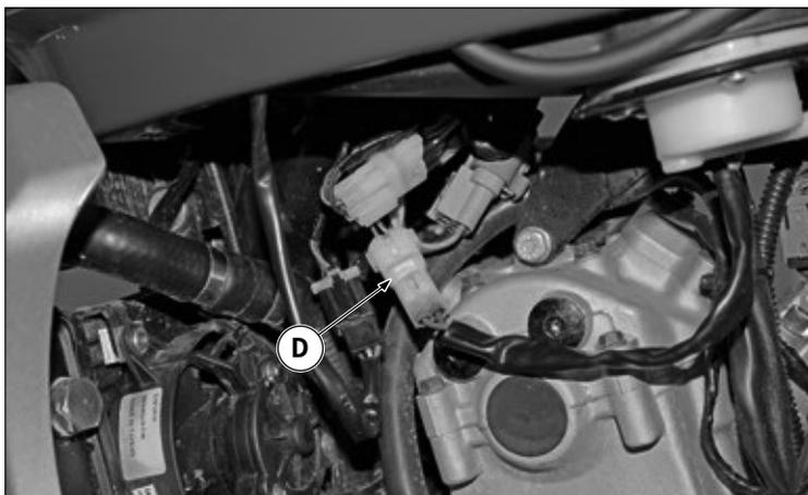
Disconnect the fuel pump connector "D" from the main wiring.
