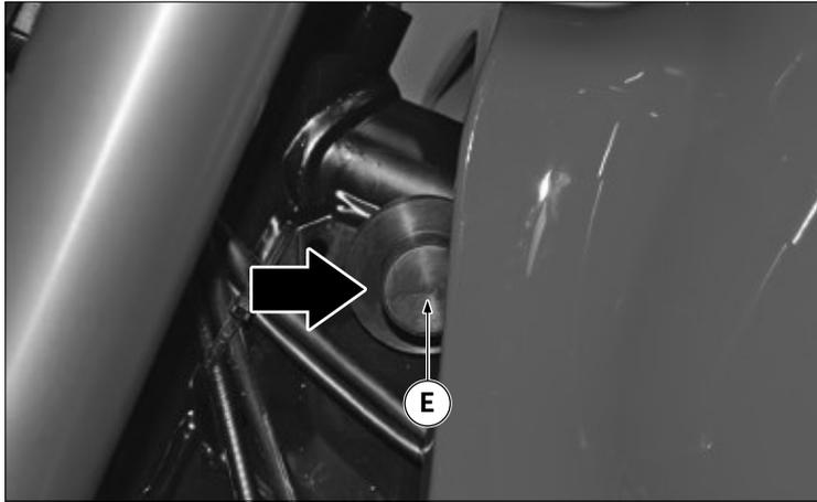
Lift the tank removing it from the front pads “E” and remove the tank.
