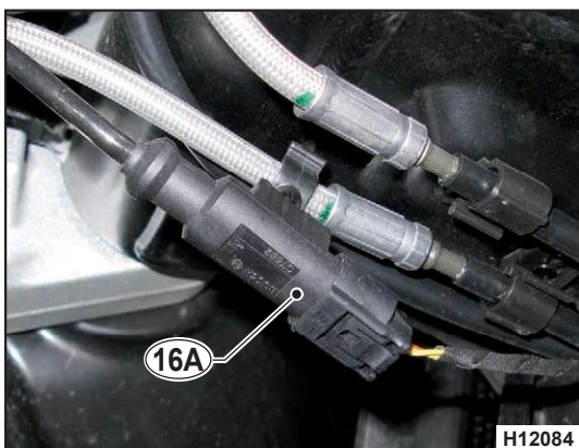
16A) Front wheel ABS sensor connector.
