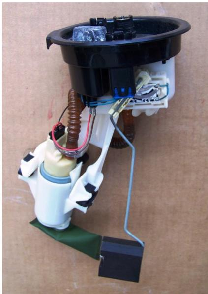
At the bottom the strainer, in the picture green, above the fuel pump and on top of it the cyclone unit
