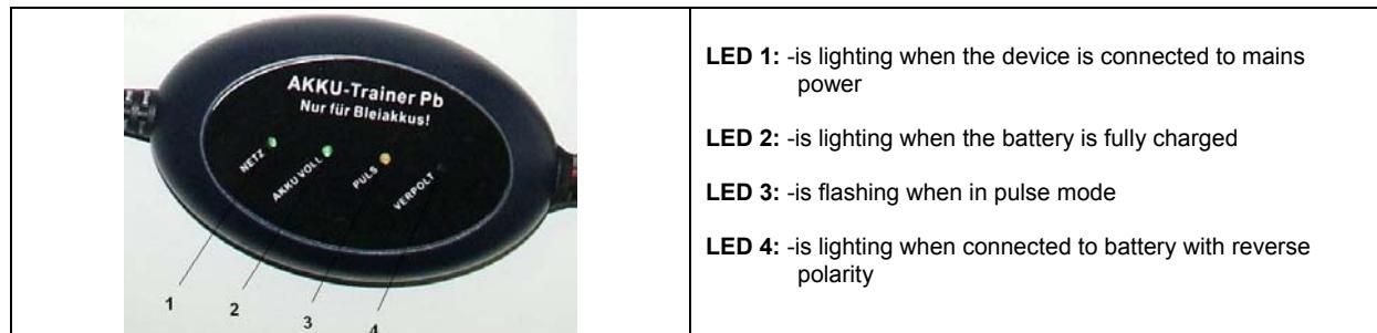
**LED 1:** -is lighting when the device is connected to mains power
